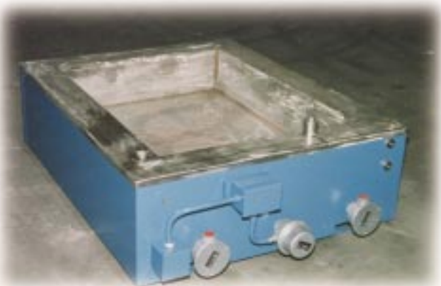
Rectangular Hot Melt Tank with “double tank” construction and a special heat transfer liquid in the outer tank which allows temperature control to \pm 2 degrees.
