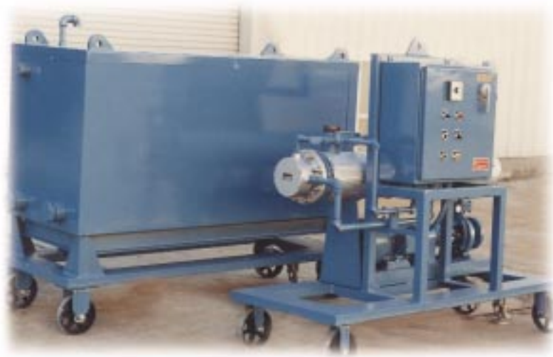
Oil Separator Heater System designed to be easily moved between locations. Note dual skid arrangement with pump skid recirculating liquid through the heated tank skid.
