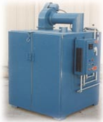
This walk-in oven measuring 6 ft. wide x 6 ft. long x 6 ft. high reaches temperatures of 600° F. with 60 kW of electric power. The recirculating ductwork on the top was unique to this application.
