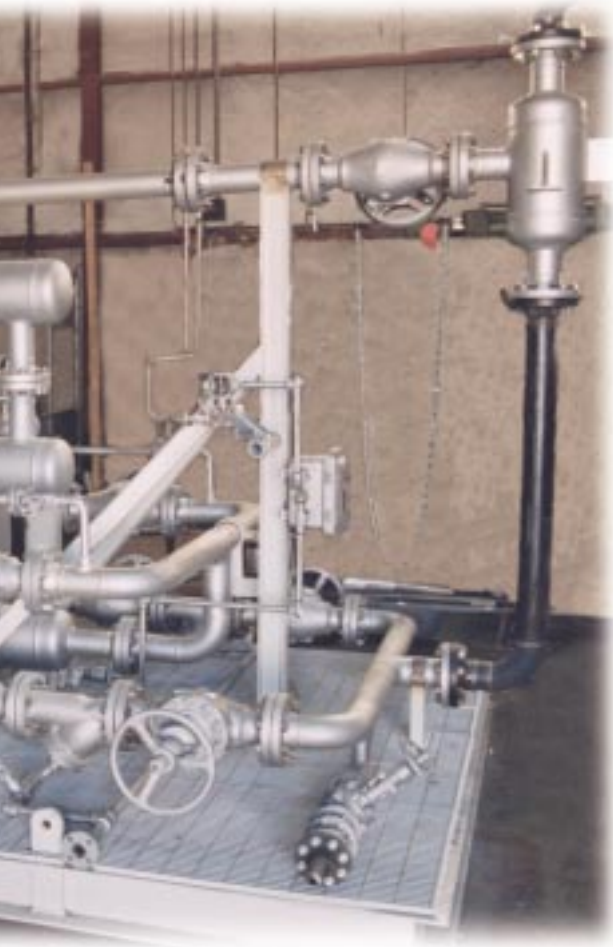
400 kW Hot Oil System designed for continuous operation in a petrochemical plant at 650° F. System was designed for installation in a hazardous location and included magnetic drive type pumps.
