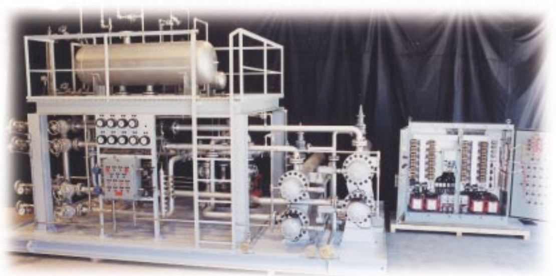
800 kW dual zone Hot Oil System for use on an extruder. System included canned motor pumps. Skid was designed for Class I, Division 2 hazardous location. Control panel remotely mounted in a non-hazardous area.
