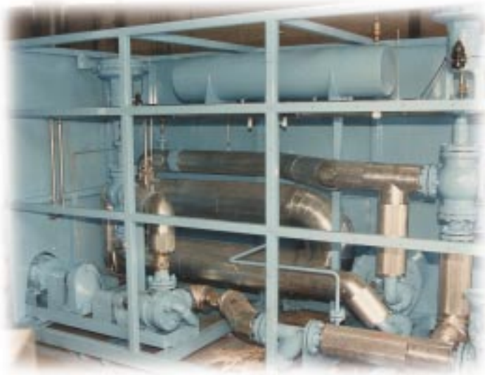
Modified GLOS Hot Oil System with an oversized expansion tank to accommodate the large volume of the customer's system. Temperature control valves were included for flow modulation to multiple zones.
