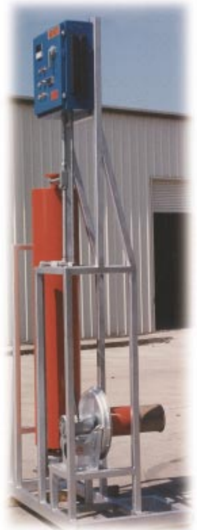
High-pressure impingement system designed for heating air from ambient to 600° F. against 26 inches of water static pressure. Assembly designed to mount below grade with control panel assembly at eye level above grade.
