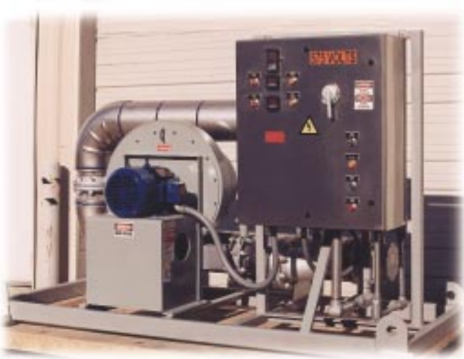
Small electric heated recirculating system capable of heating 500 SCFM air to 500° F. against 12 inches of water static pressure. System was run-tested at field conditions prior to shipment.
