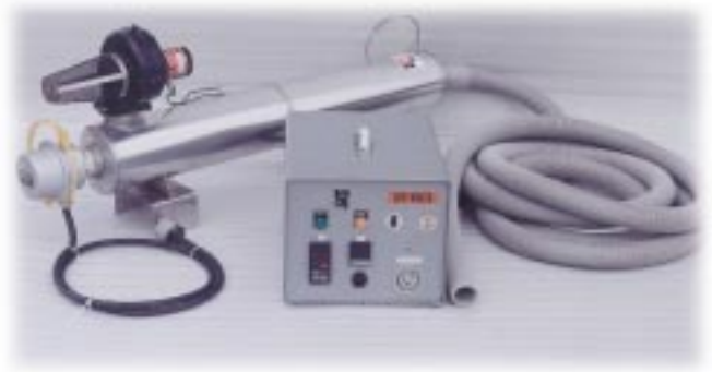
Custom-made "hot air gun" capable of accurate temperatures at higher static pressures than is found in the off-the-shelf type unit.
