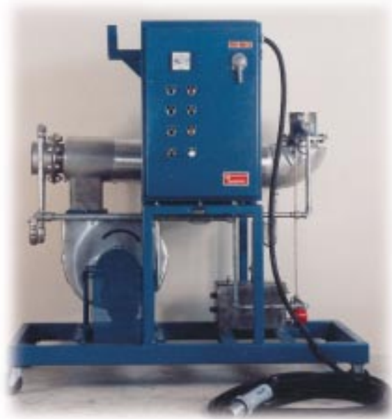
Recirculating heating-moisturizing system designed to provide 300 SCFM air between ambient and 130° F. System included a Gaumer-designed humidifying chamber capable of adding sufficient water to maintain a controlled 50%-100% relative humidity.
